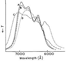
FIG. 1. Absorption spectra of (A) [CoCl<sub>4</sub>]<sup>2-</sup> in nitromethane containing 0·1M-Ph<sub>3</sub>MeAsCl, (B) [CoCl<sub>4</sub>]<sup>2-</sup> nitromethane solution, in C) Diffuse reflectance spectrum of  $Cs_3CoCl_5$ , and (D)  $[CoCl_4]^{2-}$  in dimethylformamide.
