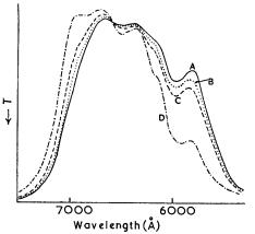
FIG. 7. Absorption spectrum of anhydrous cobalt chloride in ligroin solution containing 1% of dimethylformamide: (A) pure solvent; (B-D) added chloride, (B) 10<sup>-5</sup>M, (C) 10<sup>-4</sup>M, (D) 10<sup>-3</sup>M.
