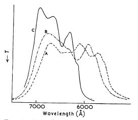
FIG. 4. Absorption spectrum of anhydrous cobalt chloride in dry nitromethane.
