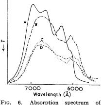
FIG. 6. Absorption spectrum of [CoCl<sub>4</sub>]<sup>2-</sup> in (A) dichloromethane, (B) dimethylacetamide, (C) dimethylformamide, and (D) dimethyl sulphoxide.
