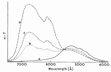
FIG. 3. Absorption spectrum of  $4 \cdot 4 \times 10^{-3}$ M-[Co(DMF)<sub>6</sub>](ClO<sub>4</sub>)<sub>2</sub> in 9:1 dimethylformamide-nitromethane containing added chloride of concentrations (A) 0, (B) 1·2, (C) 1·8, and (D)  $4 \cdot 2 \times 10^{-3}$ M.
