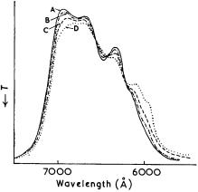
FIG. 2.  $[CoCl_4]^{2-}$  in solution in 4:1nitromethane-dimethylformamide, containing added chloride of concentrations (A) 0.2, (B) 0.4, (C) 0.6, and (D)  $0.6 \times 10^{-2}$  M.
